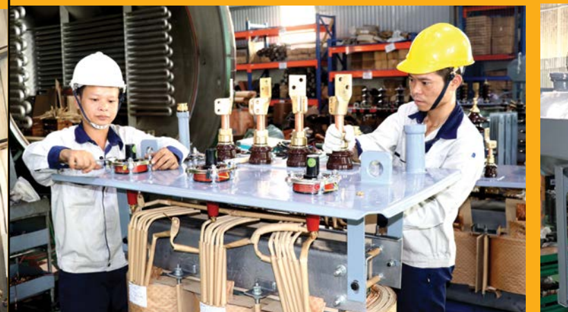
Lắp ráp MBA/Final Assembling
